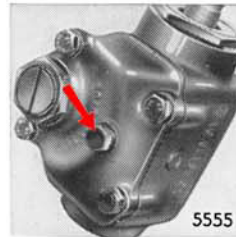
Steering case - oil filler screw
